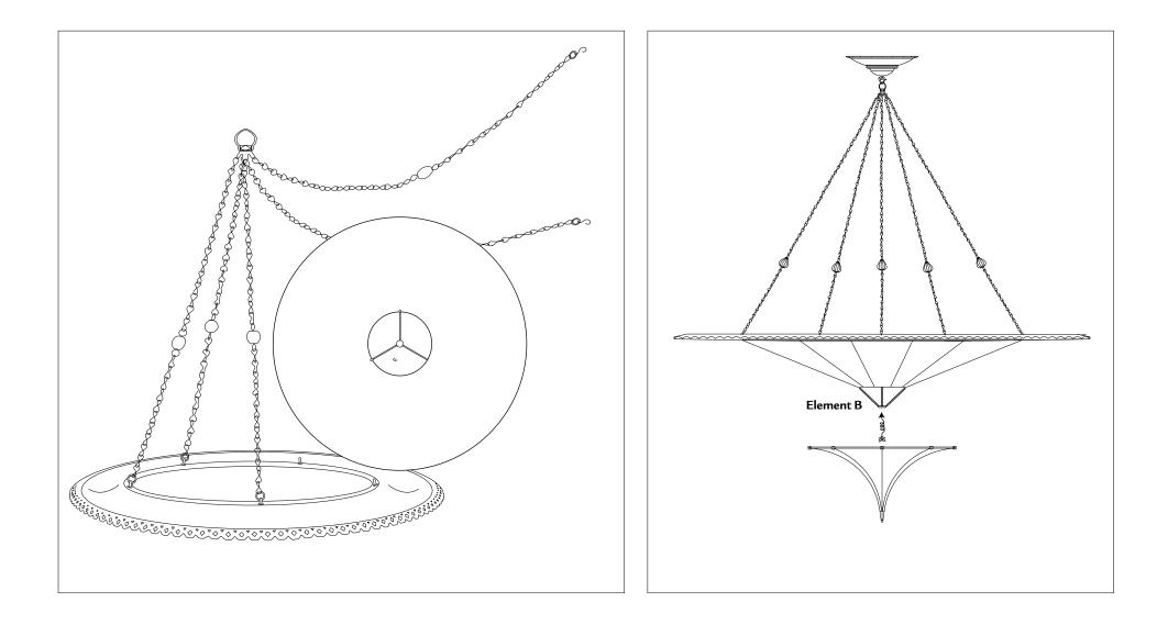
Connect the medium disk with small disk using the set of cords provided. To attach medium disk to small disk, pass the cord through the pearls following the path of the arrows (---) and then make a knot.
