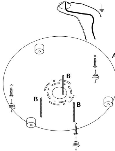
3. Make the electrical connections. Refer to the section titled Electrical Connections. Place the cover **C** over the cross bar, so that the 3 nipples **B** extends through the 3 holes cover **D**.
