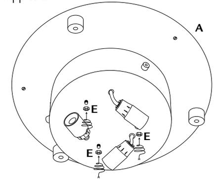
5. Install bulbs. Do not exceed the maximum wattage for this fixture. Refer to the wattage warning label attached to the fixture for maximum allowable wattage.
